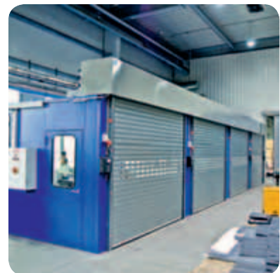
4-grinding cabin with roll-up doors
