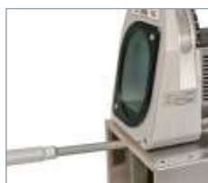
Precise adjustment of the electrode's stick-out.
