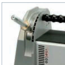
Grind the electrode in the desired angle.
